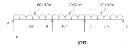
8. Analyze the beam shown in fig. using slope – deflection method and draw S.F.D. and B.M.D.
